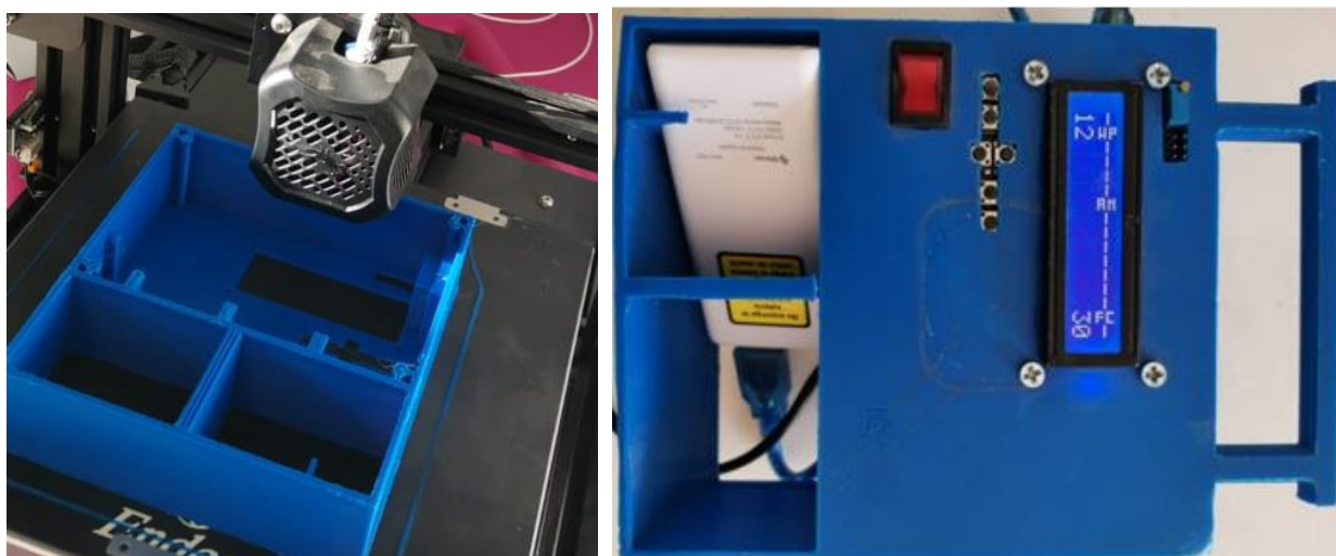
Figure 6 Printing the Device Shell (Right) and the Elaborated Prototype Showing the “Field Capacity -FC-, Permanent Wilting Point -WP- and Actual Moisture -AM- Levels” Screen (Left).
