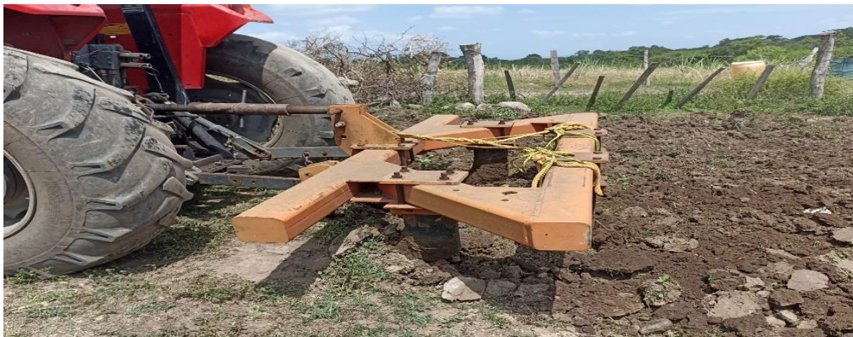
Fig. 3 Prototype Descompactor for deep soil tillage panoramic view of the prototype under real operating conditions.
