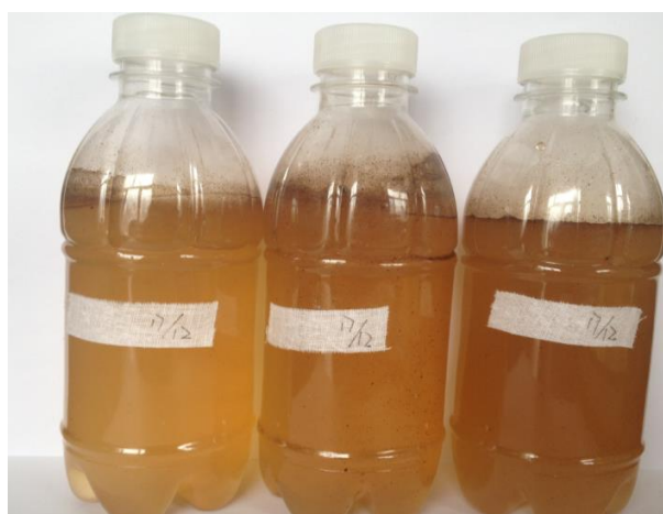
Fig. 6 Centrifugation test of produced water containing fracturing fluid.
