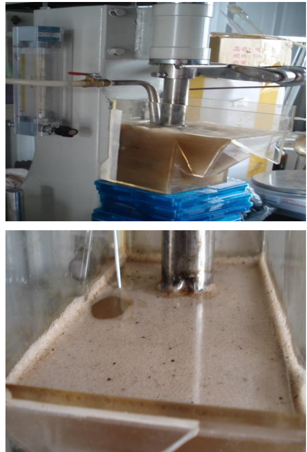
Fig. 3 Air flotation test picture of produced water containing fracturing fluid.
