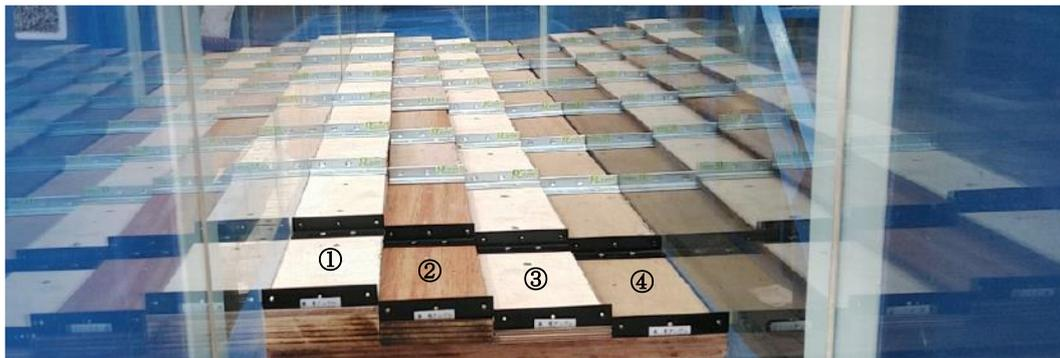
**Photo 2** Stepped channel with end sill (transverse slope:  $I_{i1} = 1/7$ ,  $I_{i2} = 1/10$ ,  $I_{i3} = 1/9$ ,  $I_{i4} = 0$  from left to right). Transverse step: 0.1 m wide, 0.25 m long, thickness  $t_1 = 0.0355 \text{ m}$ ,  $t_2 = 0.021 \text{ m}$ ,  $t_3 = 0.011 \text{ m}$ ,  $t_4 = 0 \text{ m}$ .
