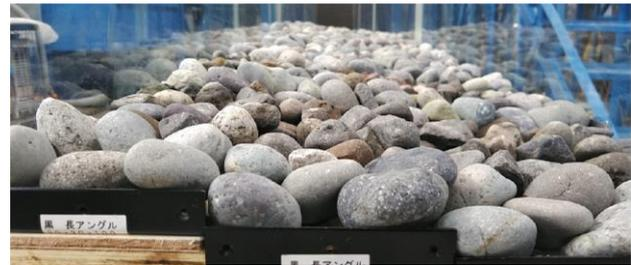
**Photo 1** Roughness slope with stacked boulders in half trapezoidal section with 1/25 longitudinal slope. Physical model with 1/10 scale was installed in rectangular channel with 0.40 m width.
