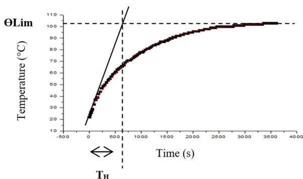
**Fig. 13 Thermal curve of the 0.75 Hp three-phase induction motor with rated load and voltage.**
