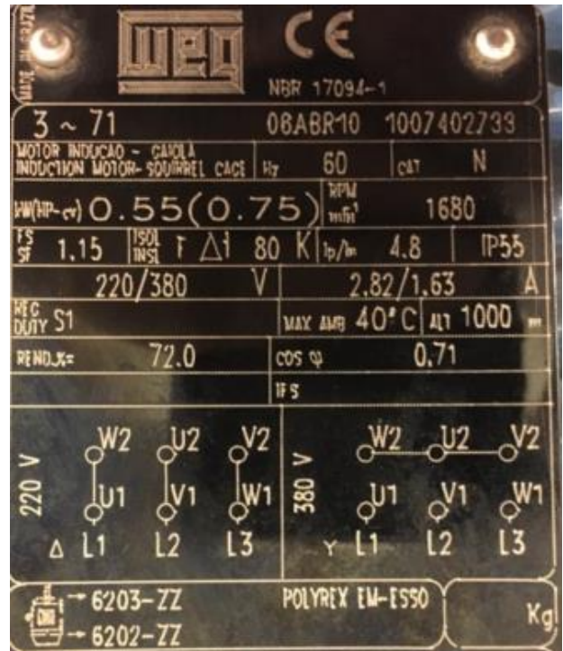
Fig. 8 Motor plate used in the SEL relay bench.
