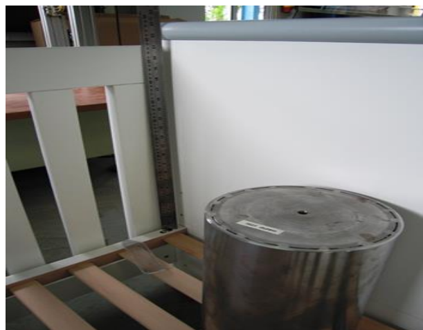
Fig. 4 Distance between footholds and top of cot sides.
