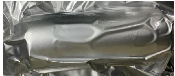
(a) Lithium metal powder container with argon gas purge
