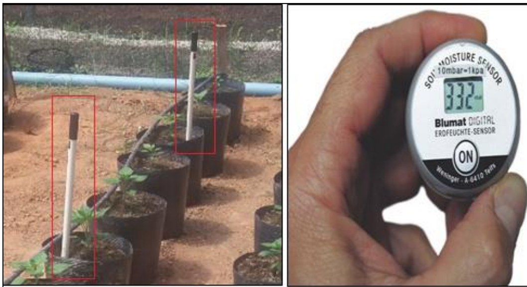
Fig. 1 Puncture tensiometers installed in the pots and digital tensiometer to obtain the tension readings.
