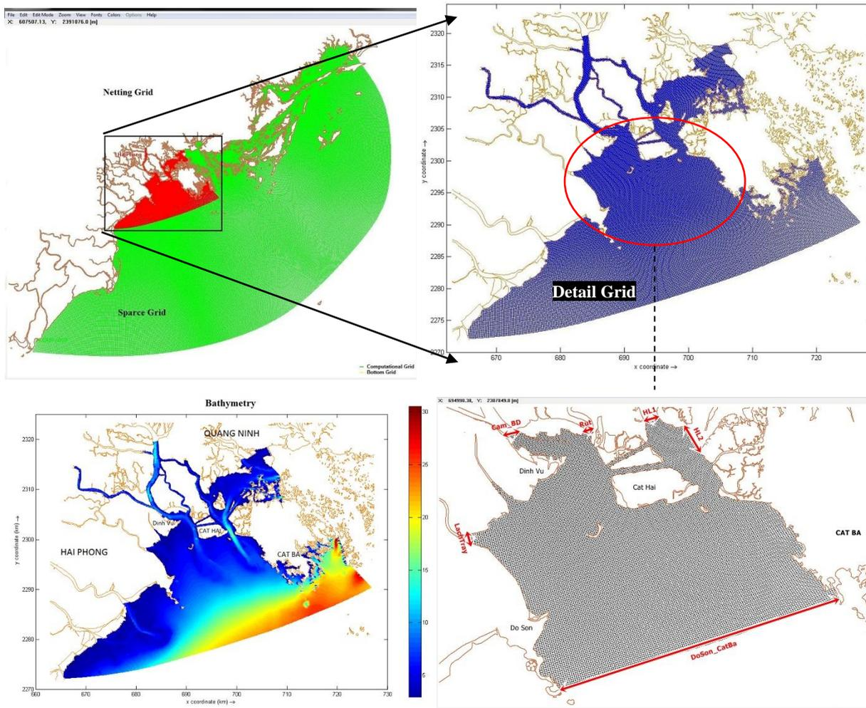
Fig. 2 Depths and grid used in the model.
