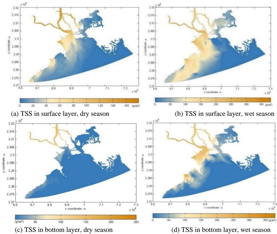
Fig. 7 Simulation results of the TSS distribution field ( $\text{g}/\text{m}^3$ ).
