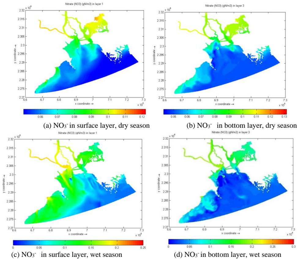
Fig. 10 Simulation results for the NO3- nutrient distribution field (gN/m<sup>3</sup>).
