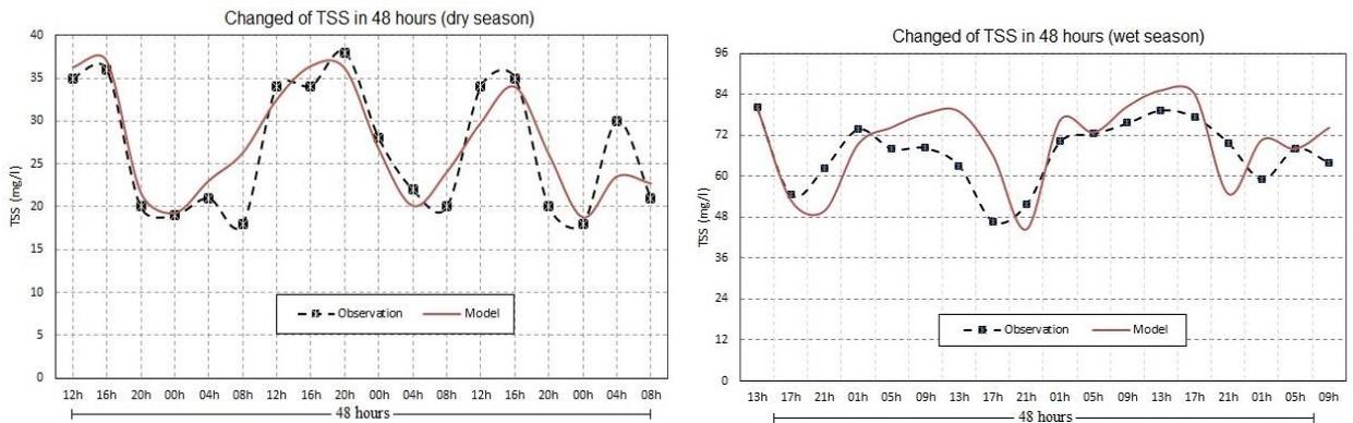
Fig. 4 TSS range in accuracy between the observed and modelled results.
