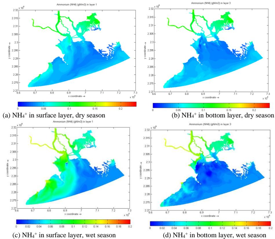
Fig. 8 Simulation results for the  $\text{NH}_4^+$  nutrient distribution field ( $\text{gN}/\text{m}^3$ ).
