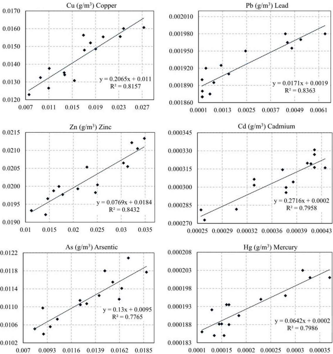
Fig. 6 Correlation graphs of heavy metals between the data measured at 15 observation points and the modelled results.
