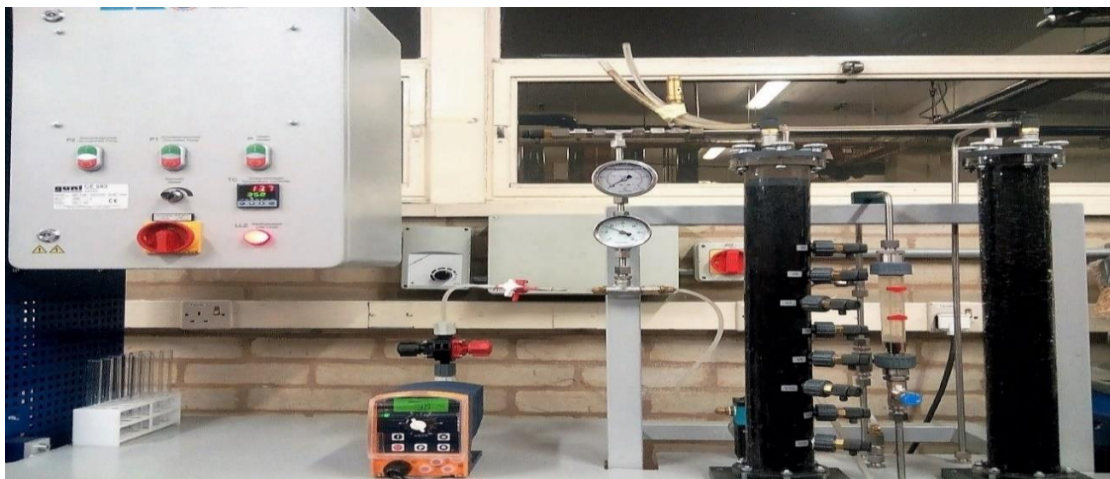
Fig. 3 Laboratory Scale testing of the rice husk charcoal filter on the CE absorption rig.
