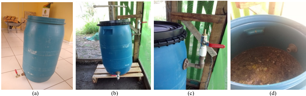
Fig. 2 a) 15° drain angle position that aids in removal of biofertilizer as it is slightly sloping downward; b) drain already applied to the plastic drum and allocated in a space reserved for the composer; c) gas outlet, relocated to the side of the plastic drum; d) distance between the gas point of outflow and the food residues (organic and nutritional). Campus VI, Paragominas - PA.
