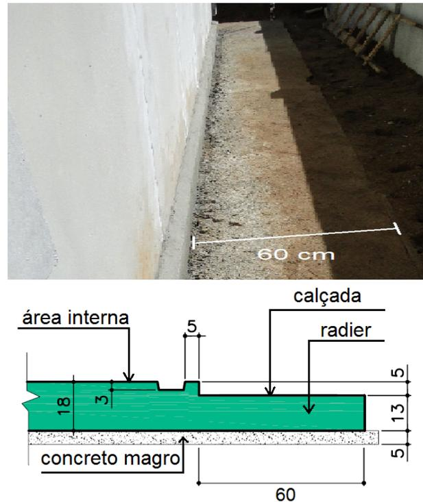
Fig. 4 Detail of the sidewalk pointing out the dimensions.
