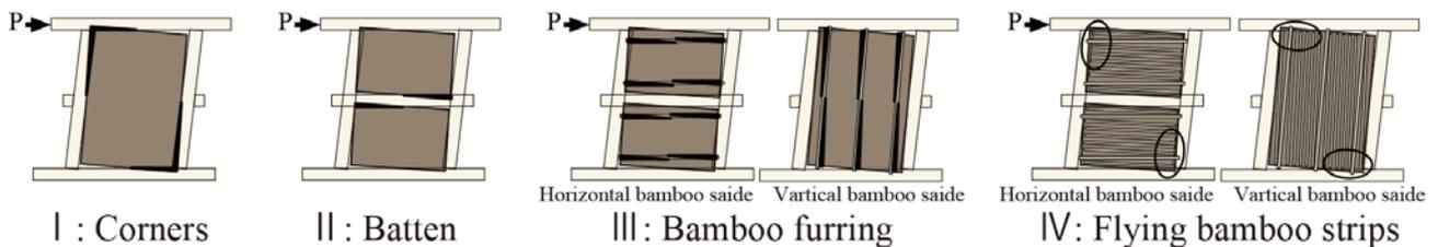
Fig. 6 Types of resistance elements.
