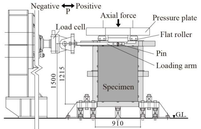
Fig. 2 Overview of the loading test apparatus.
