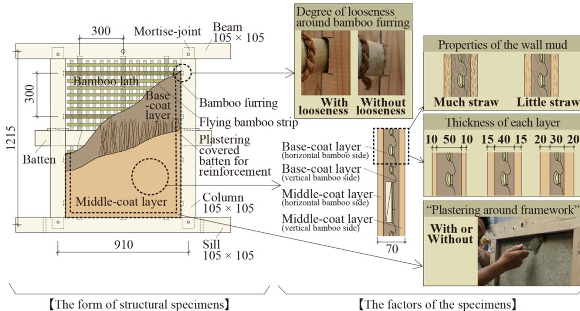
Fig. 1 Mud-bamboo wall construction for a real building and for structural specimens.
