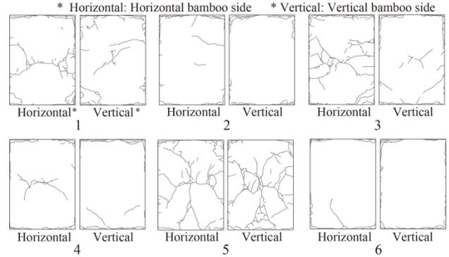
Fig. 4 State of fracture after loading test.
