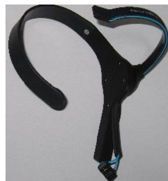
Fig. 3 Our proposed simple EEG device.
