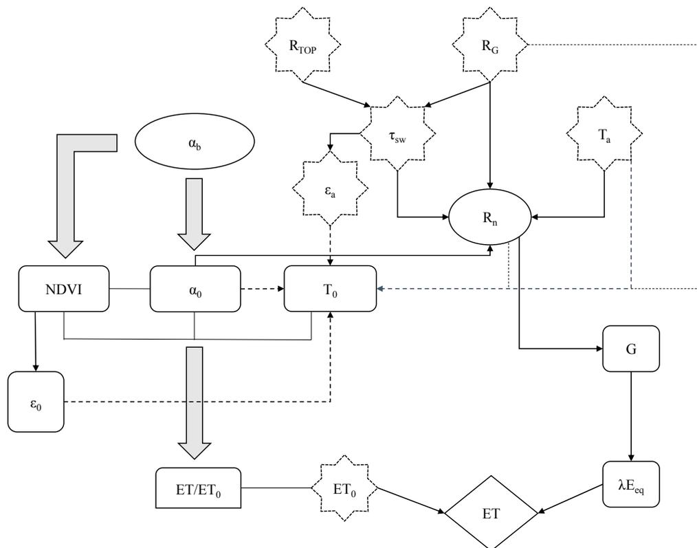
Fig. 2 Flow-chart for modelling the actual evapotranspiration (ET) throughout application of SAFER (Simple Algorithm for Evapotranspiration Retrieving) algorithm and interpolated agrometeorological data to MODIS MOD13Q1 reflectance product.
