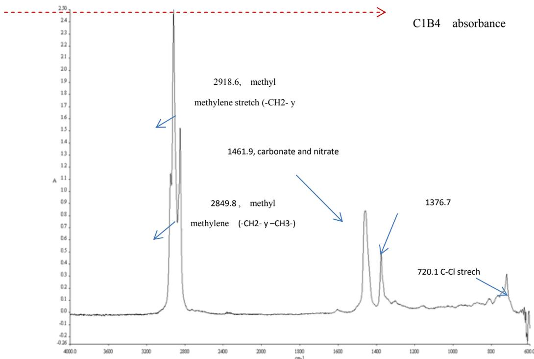
**Fig. 5 FTIR analysis C1B4 with BH.**
