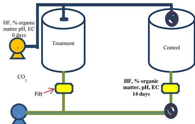
Fig. 1 Input and output variables of the coupled biostimulation, bioventing and bioaugmentation testing setup.
