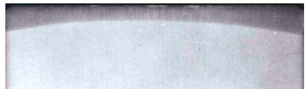
Fig. 2 Evidence of the quenched zone of a carbon steel after CSE heating and water quenching [4].
