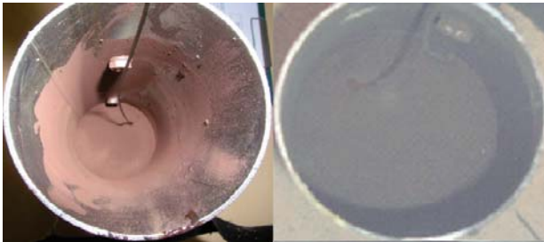
Fig. 7 Hematite to magnetite reduction using CSE [2].
