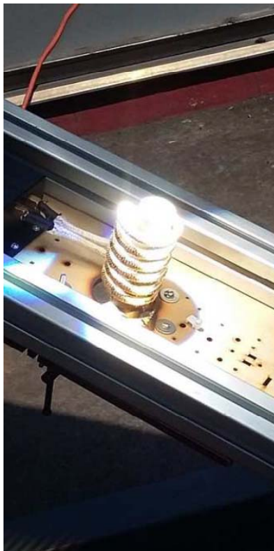
Fig. 8 Image of a hybrid induction-CSE heating system for material processing. UNAM [16].
