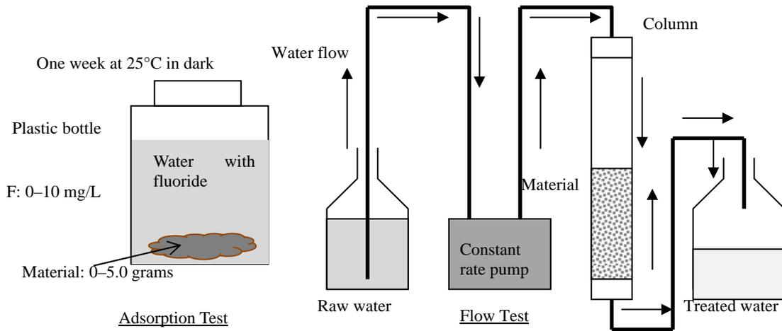
**Fig. 1 Schematic of the adsorption test and the flow test.**
