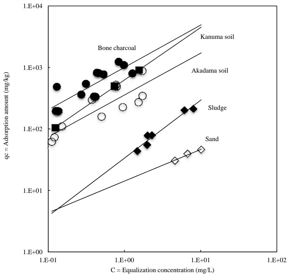
Fig. 2 Adsorption isotherm graph of adsorption tests.
