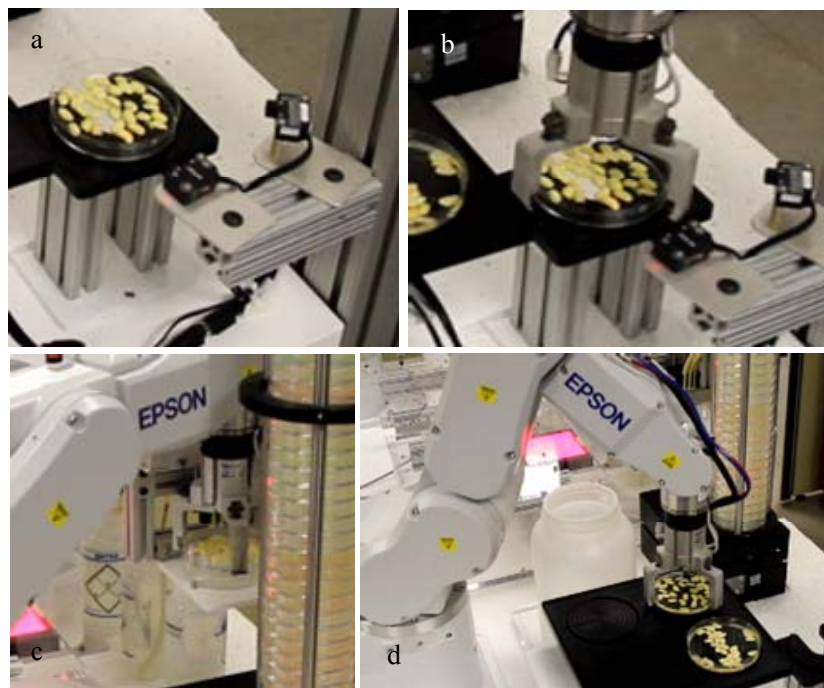
Fig. 4 a) Petri dish containing explants placed on delivery station, b) Robot A or C picking explants from delivery station c) Robot A or C places dish of explants under Agrobacterium dispensing tube, d) Robot A or C placing dish of explants onto the shaker.
