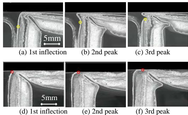
**Fig. 11 Photographs of side views of folded upper corner of Cpb2 sheets (LB160-MD120), which were scored with  $c_C = 2.5\text{ mm}$ . The fixing condition of (a)-(c) was chosen as IF+OF, while that of (d)-(f) was chosen as IF.**
