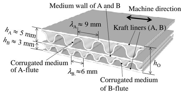
Fig. 1 Layout of double wall corrugated sheet.
