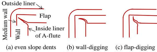
Fig. 7 Classification of folding profile of inside liner of A-flute based on observation of photo-graphs. The mode of even slope dents was detected in case of deep scoring. Two modes of wall-digging and flap-digging occurred when the scoring was insufficient with respect to the medium wall and corrugated medium of B-flute.
