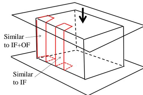
Fig. 5 Physical meaning and roles of IF and OF in the compressed panel. When seeing the middle of wall panel, the outside of wall panel is not restricted, while the left side or right side of wall panel is restricted by the corner of wall panel.
