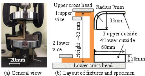
Fig. 4 Compressive test apparatus. A folded AB flute sheet, of which the width was 80 mm, was formed in Fig. 2 and Fig. 3. The panel part of this worksheet was setup in the vertical direction with the height of  $L = 83 \text{ mm}$ , and the 1st and 2nd vices clamped the upper/lower flap parts in case of IF condition. Furthermore, in case of full fixing, the OF condition was added to this IF condition.
