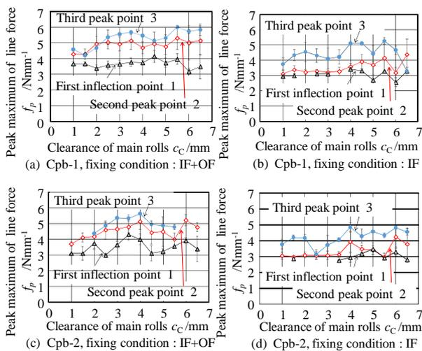
**Fig. 9 Relationship between the peak (or inflection) line force of compressive test and clearance of main rolls. Two kinds of specimens (Cpb1 and Cpb2) were arranged with two kinds of boundary constraints (IF, IF+OF).**
