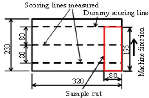
Fig. 2 Dimensions of specimen for scoring. Four samples used for folded flap-panel compressive test were cut off from a scored sheet of 320 mm  $\times$  230 mm.
