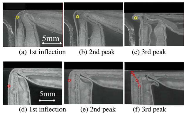
**Fig. 10 Photographs of side views of folded upper corner of Cpb1 sheets (LB210-MD120), which were scored with  $c_C = 2.5\text{ mm}$ . The fixing condition of (a)-(c) was chosen as IF+OF, while that of (d)-(f) was chosen as IF.**
