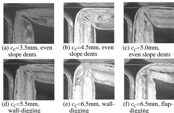
Fig. 6 Side views of upper folded corner of Cpb1 (LB210-MD120) at the initial set-up in compressive test apparatus. The fixing condition IF+OF was illustrated.
