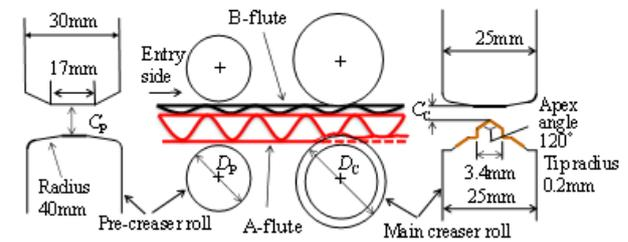
Fig. 3 Schematic diagram of scoring (lateral-creasing) apparatus. A corrugated sheet of 320 mm  $\times$  230 mm was scored by using a set of pre-creaser and main-creaser rolls in three lines with distance 80 mm apart. The main creaser roll gap was set as  $c_C$ , while the pre-creaser roll gap was set as  $c_P > h_0$  (height of sheet).
