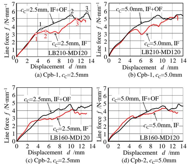
Fig. 8 Relationship between compressive line force and displacement of cross head. The first inflection point was denoted as 1. IF (inside fixing) condition was plotted as red curves, while the both side restriction, IF plus OF (outside fixing) condition, was shown as black curves. The second and third peak maximum points were denoted as 2 and 3, respectively.
