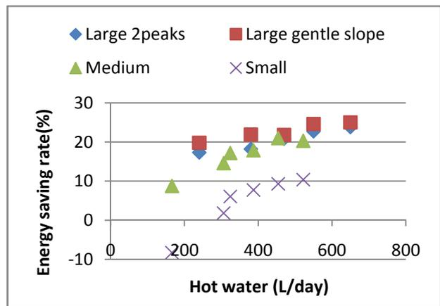
Fig. 9 Energy-saving rates with various loads.
