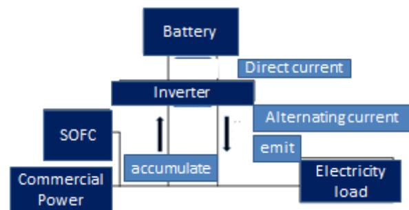
Fig. 13 Mechanism of SOFC + battery system.
