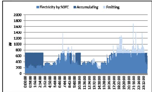
Fig. 7 Supply of electric power (medium load).
