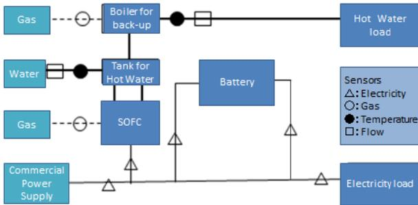
Fig. 3 System of SOFC and battery.
