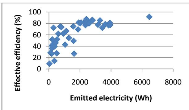
Fig. 11 Battery's trait (emission vs accumulation).
