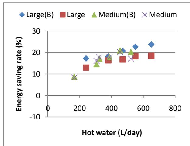
Fig. 10 Energy-saving rates (SOFC + battery vs SOFC).
