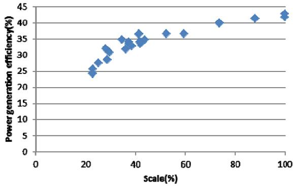
Fig. 1 Power generating efficiency of SOFC.
