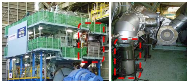
Fig. 6 Adaptation of the LP-EGR to the 4UE-X3, Demister (left), Venturi (right).
