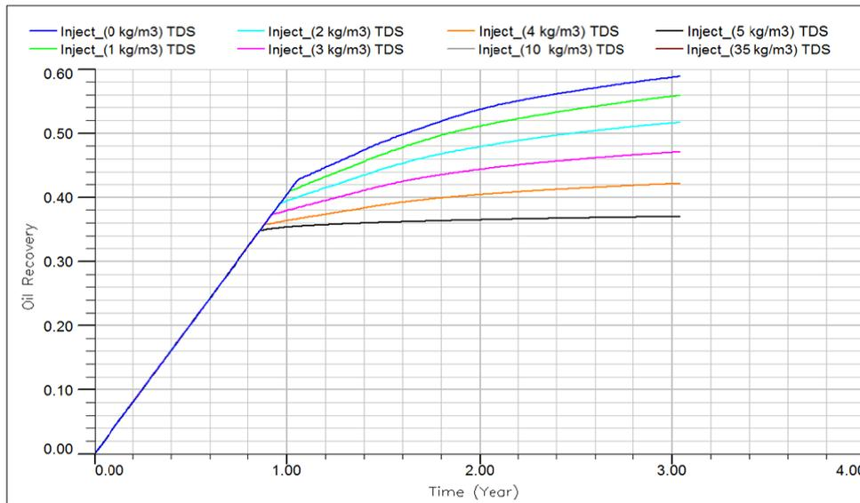
Fig. 3 Field oil efficiency (FOE) with brine salinities of 35, 10, 5, 4, 3, 2, 1, and 0 kg/m<sup>3</sup>.
