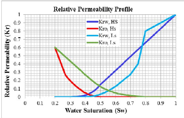
Fig. 2 Relative permeability profile for high and low salinities [16].
