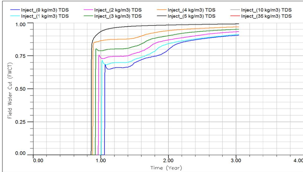
**Fig. 4 Field water cut (FWCT) with different brine salinities injection.**
