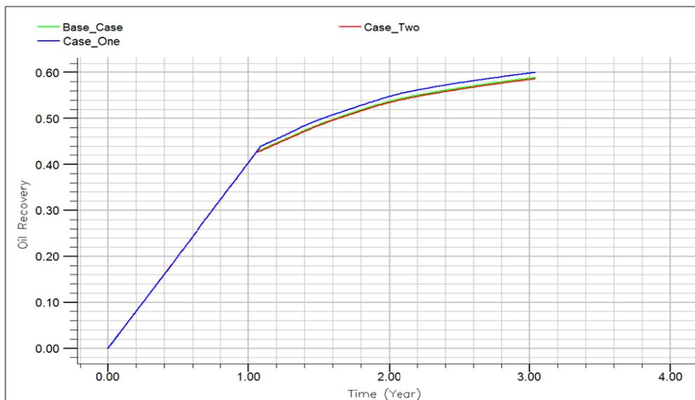
**Fig. 6 Illustrates the oil recovery for different low-salt weighting factors versus.**
