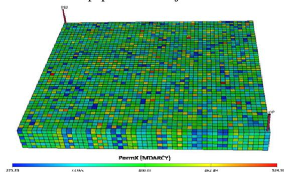
**Fig. 1** Permeability distribution and well placement in synthetic model.
