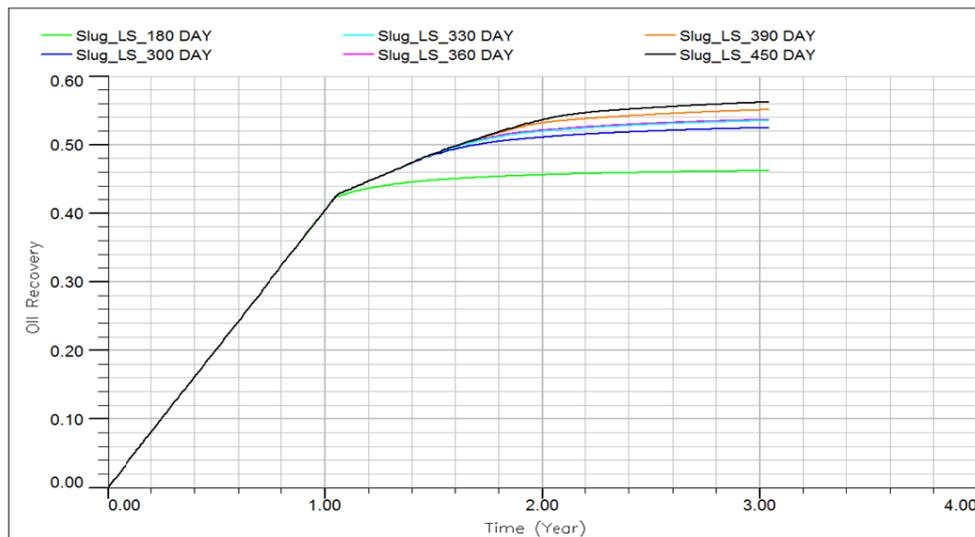
**Fig. 5 Oil recovery for different slug sizes during low salinity injection with brine salinity of 0 kg/m<sup>3</sup> TDS.**
