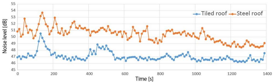
Fig. 4 Level of rain noise as a function of time.
