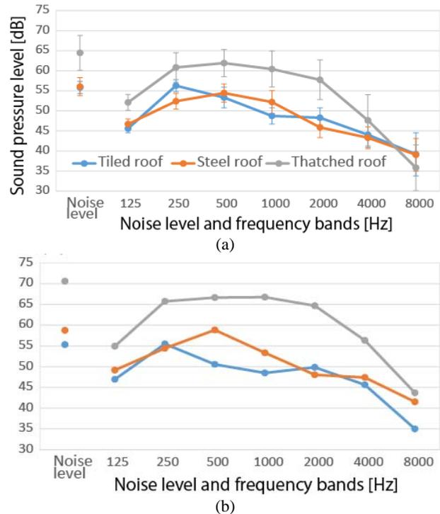
Fig. 3 (a) SPLs averaged over all sound source positions and (b) SPLs for the center source position (s5).
