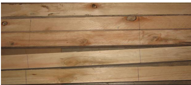
Fig. 1 Test specimens with visible knots.
