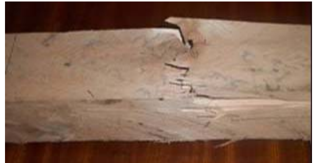
Fig. 4 Failure under flexural loading often occurs at a knot position.
