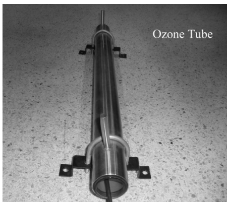
Fig. 4 The structure of ozone tube.
