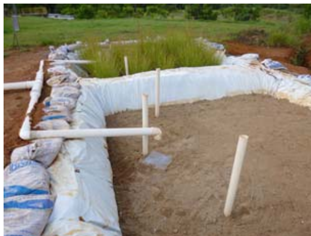
Fig. 1 Constructed Wetland Experimental Cells for Treating SW
