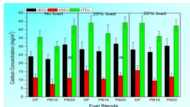
Fig. 5 The carbon content of PM emitted from diesel exhaust.
