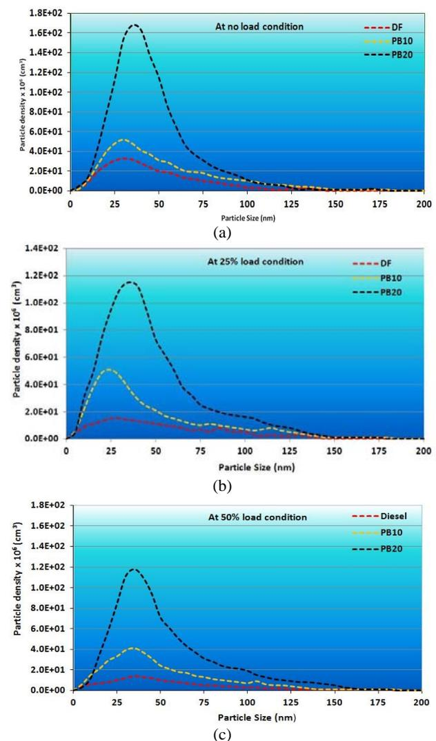
**Fig. 2** Emission concentration of the particle size and number distribution.
