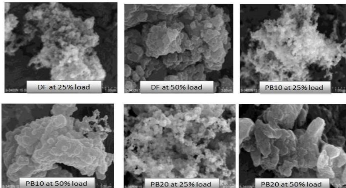
Fig. 7 SEM images for all particulate samples.
