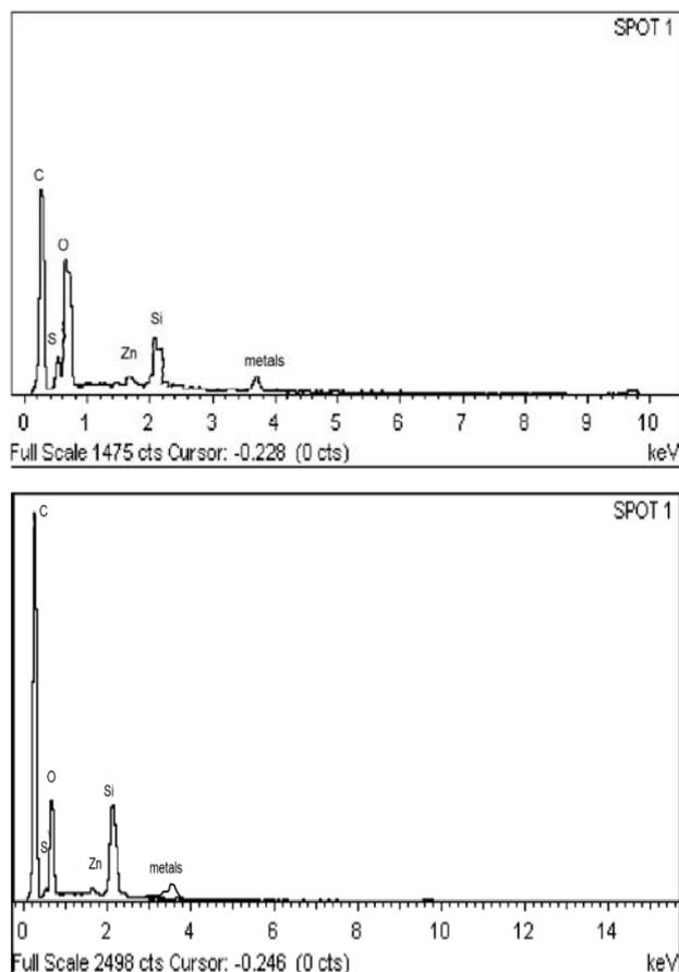
**Fig. 6** Elemental analysis for a) diesel (b) biodiesel particle matter.
